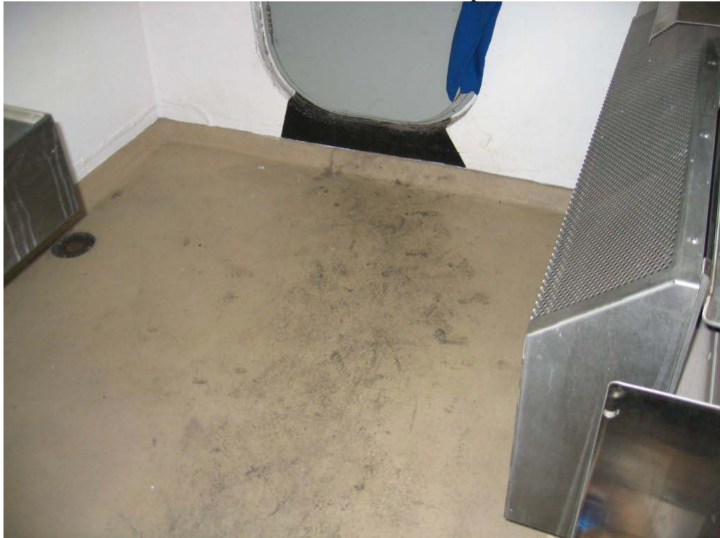
Catapult maintenance is hard, dirty work. The mild texture of this deck coating aids traction with greasy soled work boots
